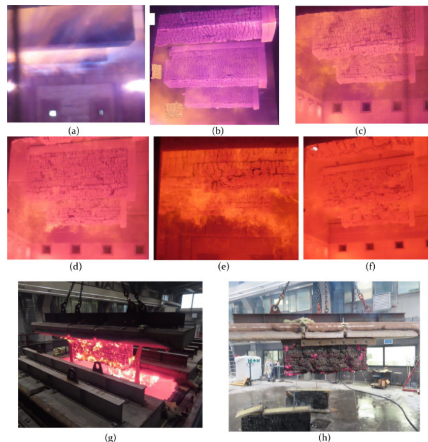
Figure 9. Fire-exposed sides of Glulam beams at test time: (a) 1 min and 50 s; (b) 22 min and 14 s; (c) 52 min and 56 s; (d) 69 min and 10 s; (e) 81 min and 46 s; (f) 115 min and 40 s; (g) 1 min and 26 s after the test; (h) 16 min and 26 s after the test [61].
