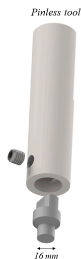
Figure 2. Schematic representation of the pinless tool geometry, consisting of a tungsten carbide (WC) tip mounted in an H13 steel holder.
