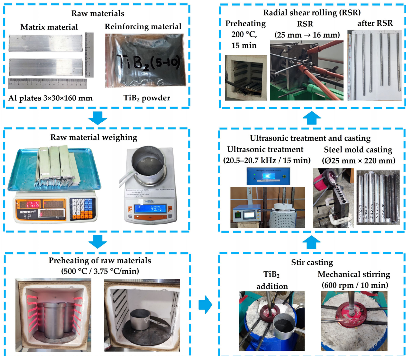
Figure 2. Schematic representation of the fabrication route for Al6060/TiB 2 composites using stir casting combined with ultrasonic treatment and subsequent radial-shear rolling (RSR).
