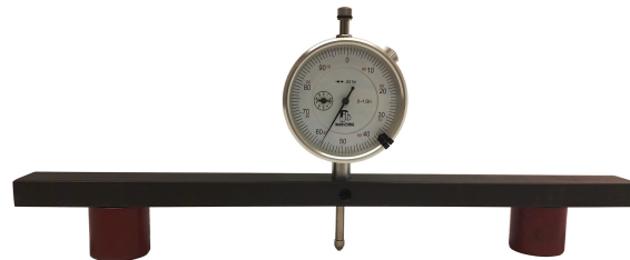
Figure 2. Piston deck height gauge measurement system used in the experiments. The measurement reading is the distance from the table to the top of the plate.
