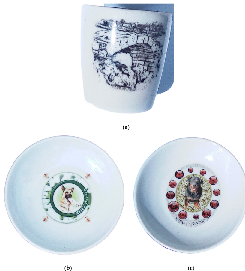
Figure 10. Microwave-fired samples in white porcelain: (a) black decal fired at 920 °C for a 50 min heating cycle; (b,c) colored and detailed decals fired for 43 min, plus a soaking time of 5 min at the maximum temperature of 1180 °C. Photos are presented with the camera flash.
