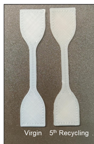
Figure 11. Virgin versus fifth recycling cycle TPE specimen.
