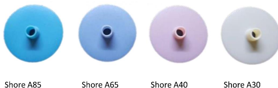
Figure 6. Valves fabricated with different combinations of two base materials to achieve different levels of hardness.
