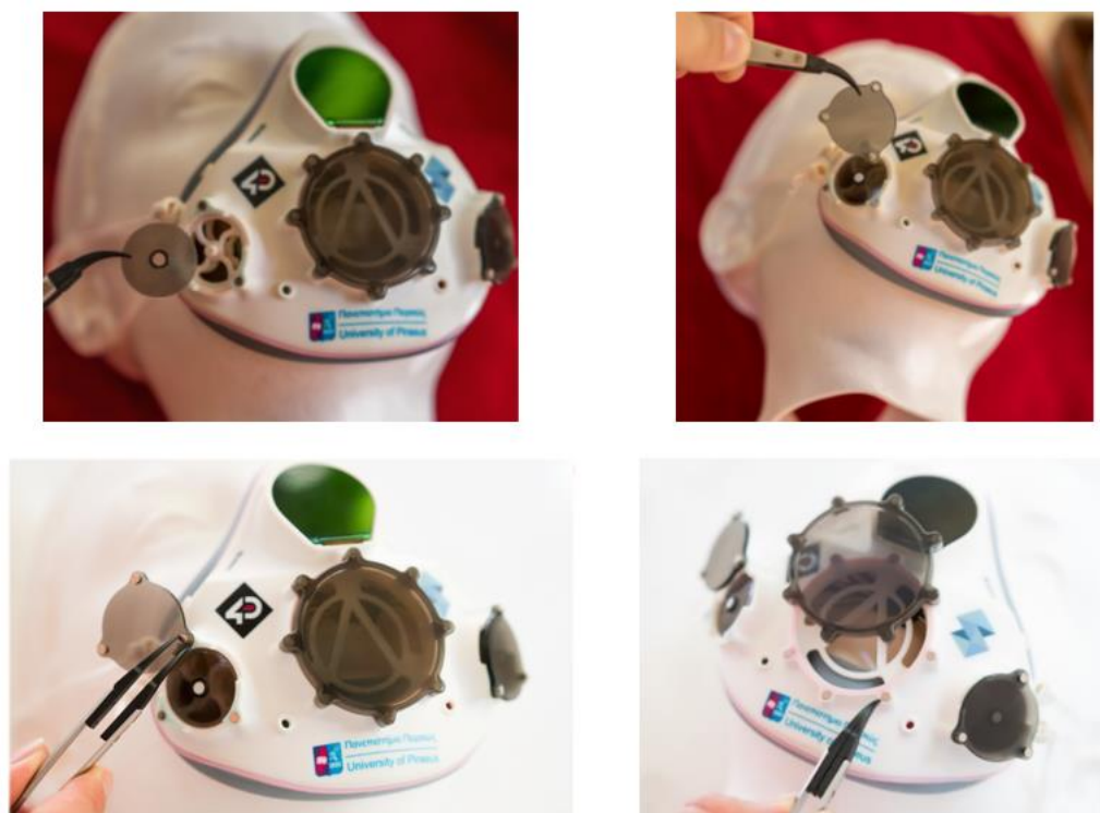
Figure 7. Assembly of the exhaust valve, main filter, and the corresponding covers on the main body.
