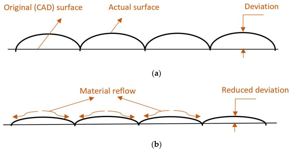
**Figure 9.** Chemical treatment mechanism: (a) before the chemical reaction and (b) after the chemical reaction.
