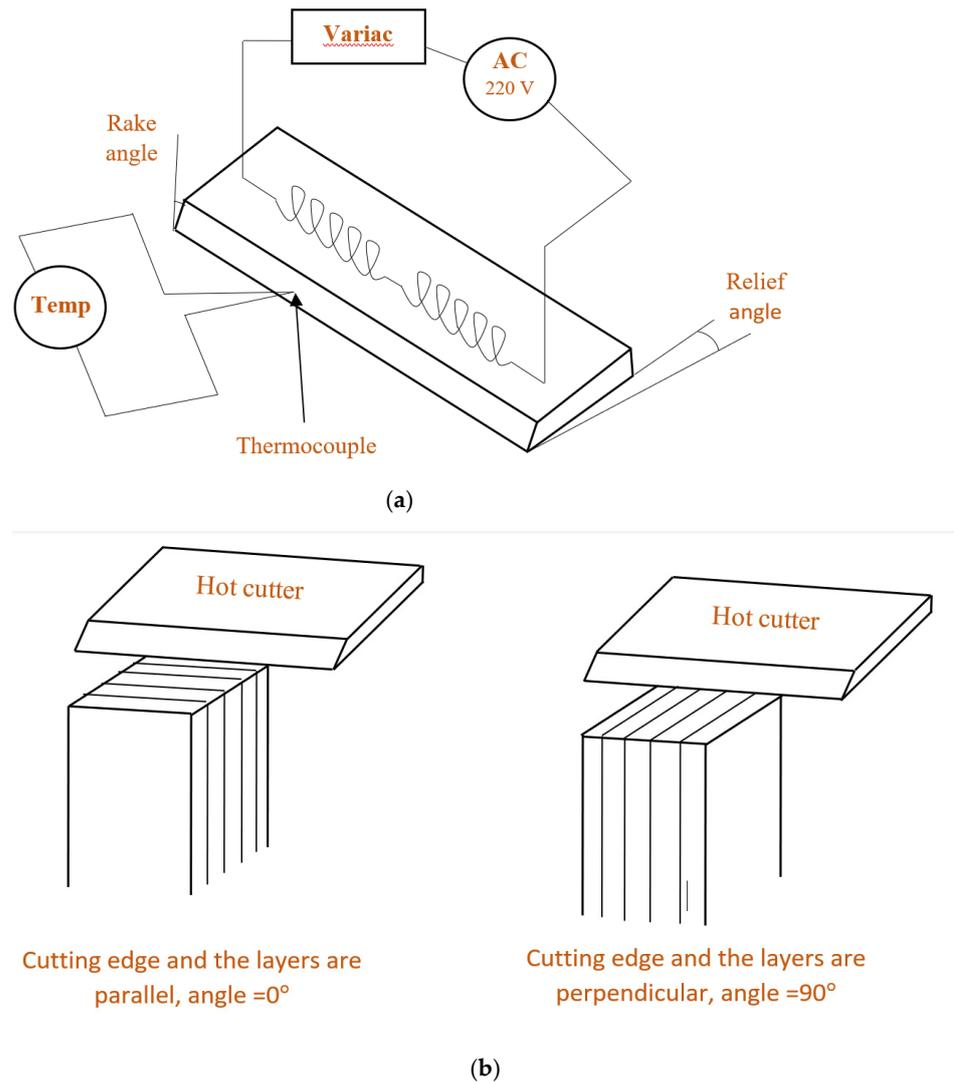
**Figure 13.** Machining with the heated cutter: (a) shape of the cutter and (b) direction of the machining.
