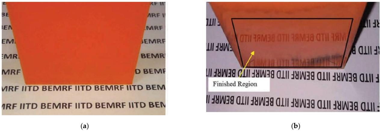
**Figure 8.** FDM-ed sample: (a) unfinished surface and (b) finished surface after applying the BEMRF process [19].
