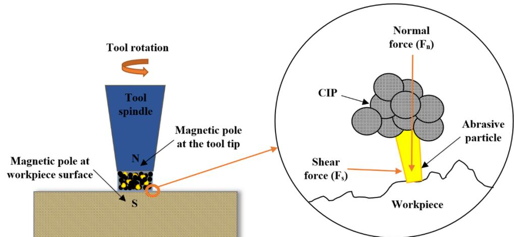
Figure 6. The BEMRF process.
