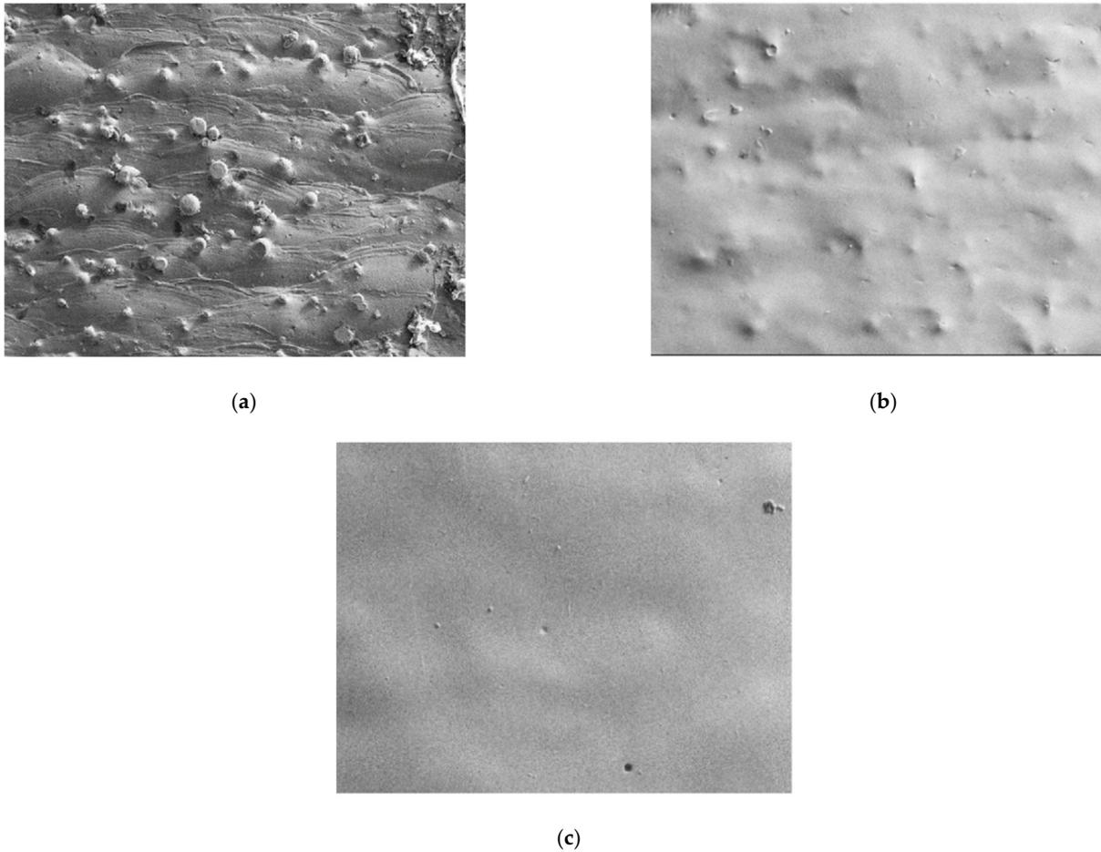
**Figure 18.** Surface of the part: (a) prior to finishing; (b) 2 min; (c) 5 min after EC finishing [67].
