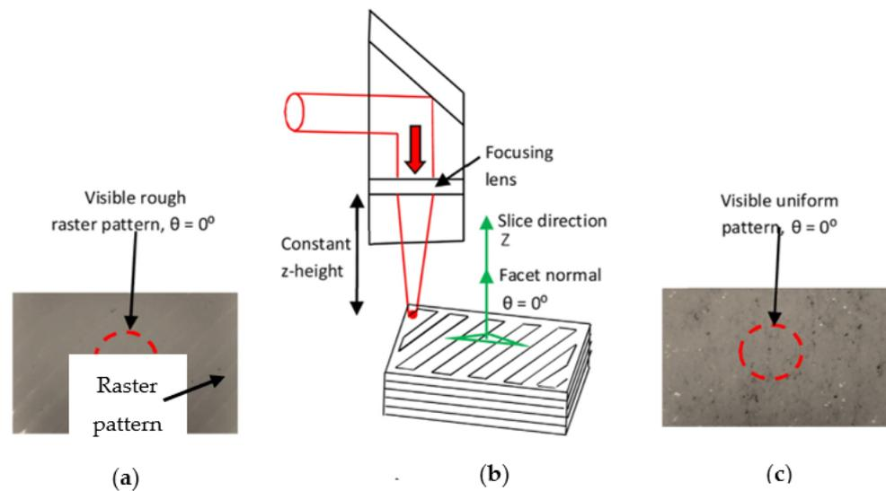
**Figure 15.** The result of laser polishing the ABS part at a build orientation angle  $\theta = 0^\circ$ : (a) raster pattern before laser polishing; (b) schematic of laser polishing; (c) laser polished surface [36].
