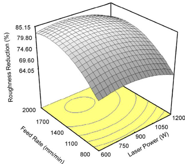
**Figure 17.** The effect of process parameters in the LF of AM parts [39].
