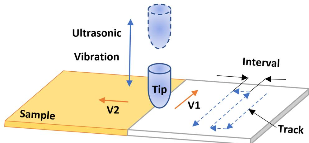
**Figure 20.** Schematic of the UNSM process.
