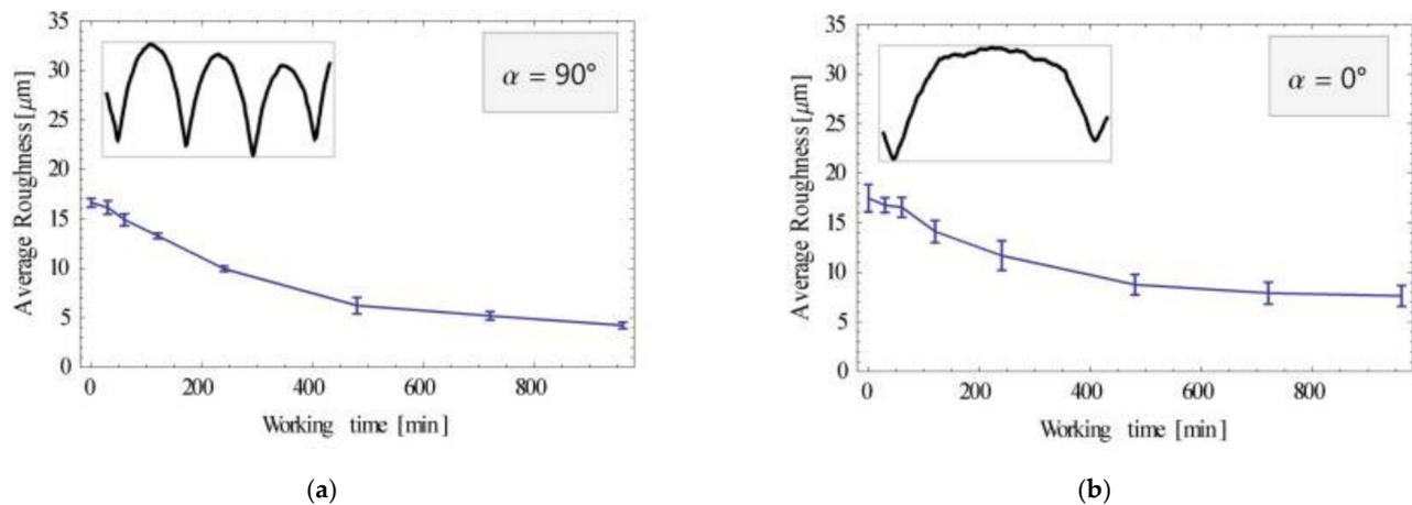
**Figure 4.** Surface roughness with the indication of the initial peaks as the function of time for: (a) the deposition angle  $\alpha = 90$  and (b) the deposition angle  $\alpha = 0$  [16].
