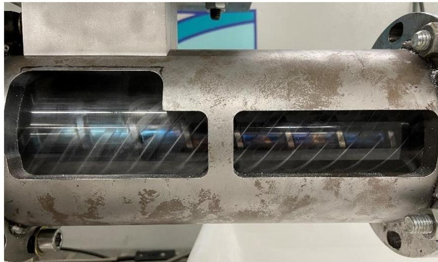
**Figure 6.** Experimental set-up using a helically grooved PMMA barrel.
