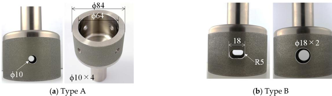
Figure 4. Configuration of grinding wheel and holes for optical path.
