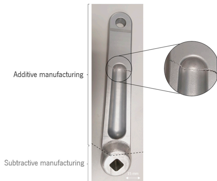
Figure 11. Hybrid crankset after the three-point flexural test.
