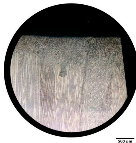
Figure 9. Cross section of in the x-z plane (x being the torch moving direction and z being the height) of the Inconel 718 30-layer wall structure.
