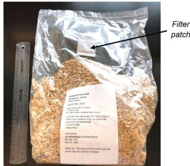
**Figure 1.** As-received biomass–fungi material in a filter patch bag.
