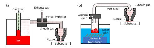
Figure 18. Schematics of (a) pneumatic and (b) ultrasonic aerosol jet printing.
