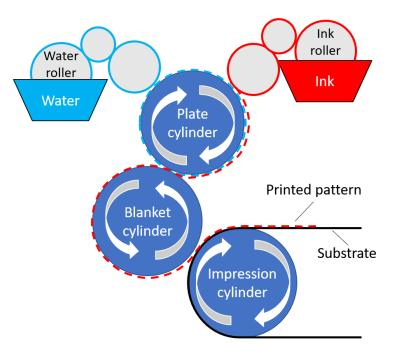
Figure 13. Schematics of offset printing.
