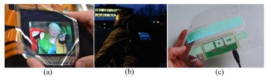
**Figure 10.** (a) A flexible color display (Reprinted with permission from [128]. Copyright 2018 IEEE); (b) a screen printed electroluminescent matrix display integrated into a back pack; (c) a closer look of the screen printed electroluminescent matrix display with the controlling module (Reprinted with permission from [129]. Copyright 2018 IEEE).
