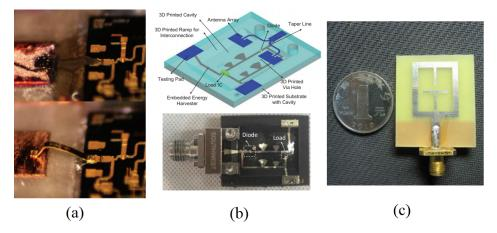
**Figure 8.** (a) Printed interconnect (above) and a ribbon-bond interconnect (below) (Reprinted with permission from [83]. Copyright 2020 IEEE); (b) the structure for the embedded-on-package 5G energy harvester (above) and printed device (below) (Reprinted with permission from [86]. Copyright 2019 IEEE); (c) Printed antenna for WLAN and 5G applications (Reprinted with permission from [84]. Copyright 2020 IEEE).
