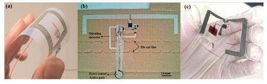
**Figure 7.** (a) A printed RFID coil by the authors; (b) a fabricated RFID tag with an opening sensor and force sensor as a part of the packaging [39]; (c) an RFID tag with light detection capabilities printed on a flexible PEN substrate [40].
