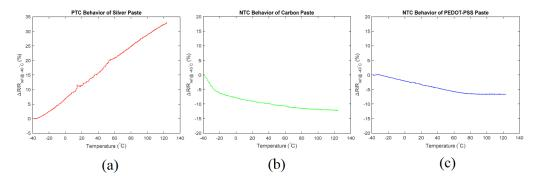
**Figure 4.** (a) Highly linear PTC behavior of silver throughout the test temperature range; (b) NTC behavior of carbon; (c) NTC behavior of PEDOT:PSS. Note that carbon exhibits near linear NTC behavior after an initial region of non-linear behavior (roughly from -40 °C to -20 °C). On the other hand, PEDOT:PSS behaves near linearly initially from around -40 °C to 70 °C. (Reprinted with permission from [50]. Copyright 2020 IEEE).
