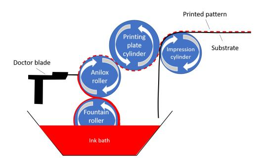
Figure 14. Schematics of flexography.
