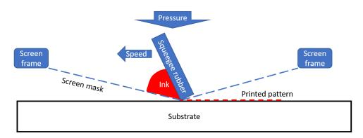
Figure 15. Schematics of screen printing.
