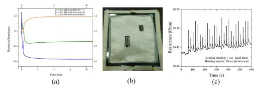
**Figure 5.** (a) Normalized impedance over time for vacuum and curing cycles for three types of resin; (b) Printed strain sensor placed on glass fiber reinforced composite; (c) Results of impact hammer bending of glass fiber reinforced composite with embedded printed strain sensor. (Reprinted from [62] under CC BY-NC-ND 4.0 license).
