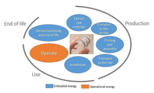
**Figure 19.** Holistic overview for life-cycle of a printed electronics device. Operational energy is the energy required to use the device while embodied energy refers to the consumed energy by the processes associated with the production and end of life.
