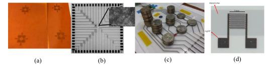
**Figure 3.** Printed sensors: (**a**) temperature sensors showing transparent property PEDOT:PSS (Reprinted with permission from [50]. Copyright 2020 IEEE); (**b**) a CNT gas sensor array; (**c**) a resistive pressure sensor array with test weights (Reprinted with permission from [13]. Copyright 2017 IEEE); (**d**) a PEDOT:PSS based temperature sensor with silver nanoparticle electrodes (Reprinted from [49] under CC BY 4.0 license).
