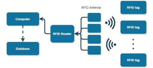
**Figure 6.** An illustration of an RFID system consisting of multiple RFID tags and an RFID reader connected to a computer managing a database.
