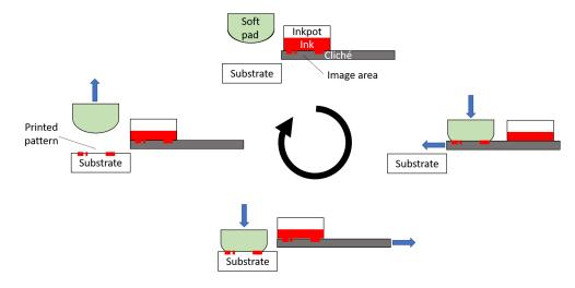
Figure 16. Schematics of pad printing.
