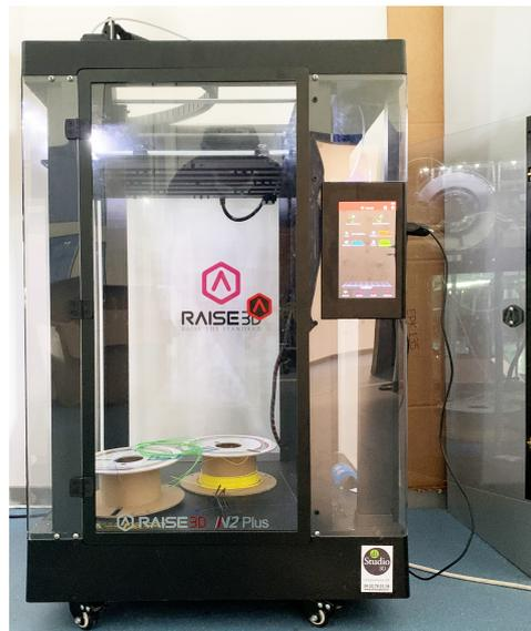
**Figure 21.** Rise 3D Printer V2 Plus used to manufacture the printed parts in Figures 15, 18 and 20.
