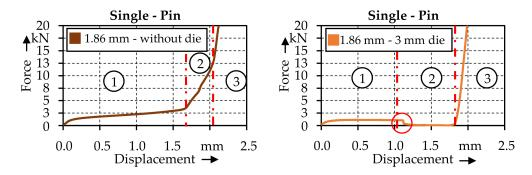
**Figure 9.** Comparison of the force displacement curves of the two investigated joining strategies based on the 1.86 mm pin structures.
