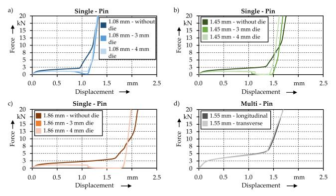
**Figure 8.** Force-displacement curves of the direct pin pressing joining process. (**a**) Force-displacement curves when joining 1.08 mm pins without and with die, (**b**) Force-displacement curves when joining 1.45 mm pins without and with die, (**c**) Force-displacement curves when joining 1.86 mm pins without and with die and (**d**) Force-displacement curves when joining 1.55 mm multi pin structures.
