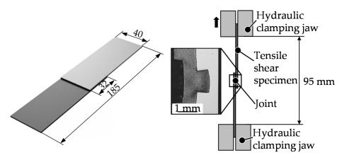
Figure 4. Schematic illustration of tensile shear specimen and test setup.
