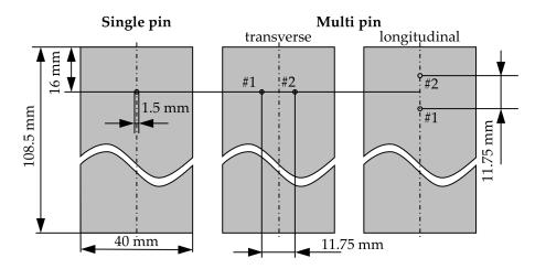
Figure 2. Schematic illustration of the investigated pin arrangements.
