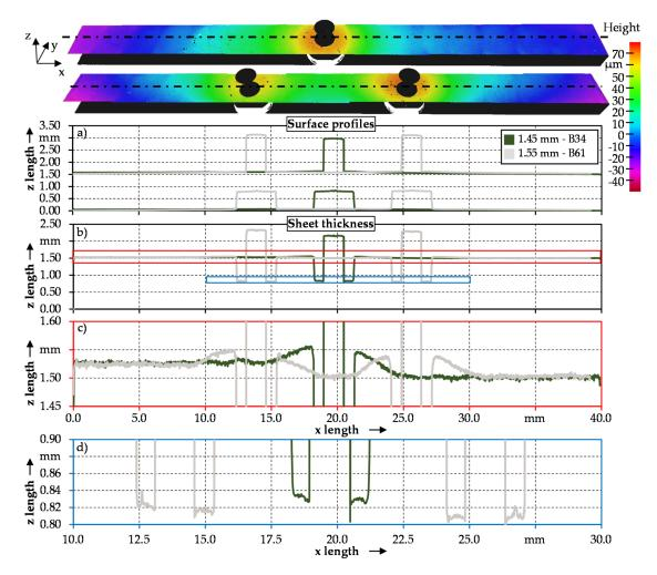
**Figure 7.** Illustration of the surface profile of a single and multi-pin structure as well as the sheet thickness across the width of the sample. (a) Surface profiles of the measured specimens, (b) corresponding sheet thickness, (c) detailed view of the red area marked in subfigure (b) and (d) detailed view of the blue area marked in subfigure (b).
