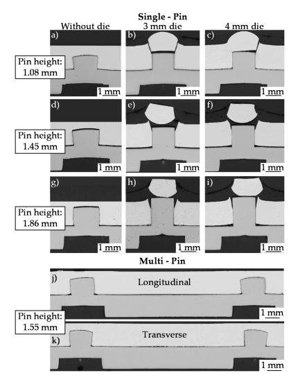
highest pin structures examined, with an average height of 1.86 mm, the compression is approximately 33% and a barrel-shaped pin can be observed.
