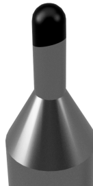
Figure 4. Appearance of the used ball radius tooling. The tip is coated.
