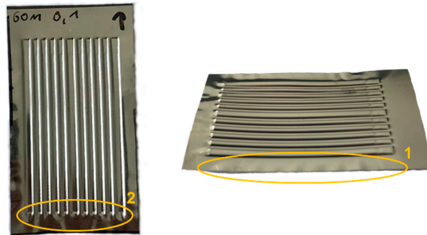
Figure 7. Experimental roll forming results. (1); wrinkles over length (2) wrinkles over width.
