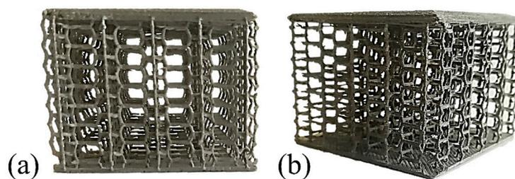
**Figure 4.** Developed manufacturing process as-cast sample ( $T_M = 250$  °C and  $T_C = 700$  °C, using vacuum assistance).
