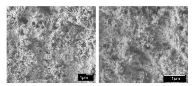
Figure 8. SEM of sol-gel-deposited CaP microstructure in different magnifications of the same area [78].
