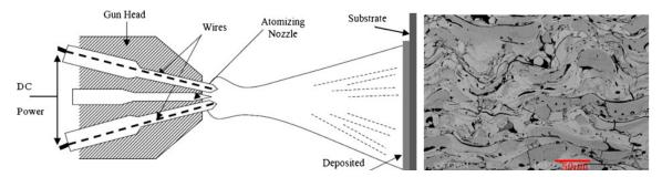
**Figure 13.** (a) Schematic arc wire spray coating setup and mechanism of operation [117]. (b) SEM micrograph of arc wire spray-coated surface by Tafa's steel (95MXC) cored wire feedstock. The substrate material is not mentioned in Reference [114].
