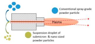
Figure 10. Schematic plasma spray coating setup and its parts [98].
