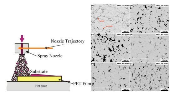
**Figure 12.** Left: A schematic of warm spray coating technique and its setup [115]. Right: Cross-section BSE micrographs of warm spray-deposited Ti-6Al-4V on low-carbon steel substrate processes spray pressure and nitrogen flow rates of (a) 1 MPa and 0.5 m3/min, (b) 1 MPa and 1 m3/min, (c) 1 MPa and 1.5 m3/min, (d) 4 MPa and 0.5 m3/min, (e) 4 MPa and 1 m3/min, and (f) 4 MPa and 1.5 m3/min, respectively [116].
