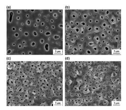
**Figure 4.** SEM micrographs of MAO coating structures under different frequencies of (**a**) 60 Hz, (**b**) 500 Hz, (**c**) 1000 Hz, and (**d**) 2000 Hz [40].
