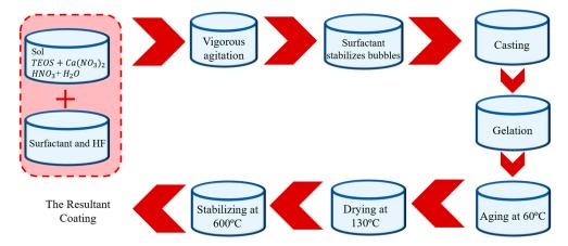
**Figure 7.** Schematic sol–gel coating process from solution preparation to the final solid structure formation.
