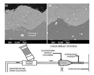
**Figure 11.** Top: SEM micrographs of cold spray-coated AA6061 substrate by (**a**) as-received and (**b**) heat-treated AA7075 particles with a mechanical interlocking between the coating and the substrate [105]. Bottom figure: a schematic view of cold spray coating process [106].
