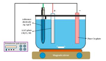
**Figure 5.** Schematic setup for electrodeposition of copper metal particles over aluminum oxide [52].
