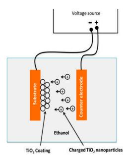
**Figure 6.** Sketch of the electrophoretic deposition process [60].
