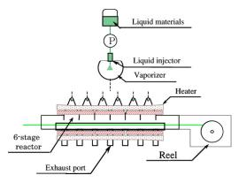
**Figure 2.** Schematic chemical vapor deposition (CVD) setup, mechanical parts, and operation mechanism [23].
