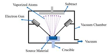
**Figure 1.** Schematic view of a physical vapor deposition (PVD) machine using electron beam as the heat source.
