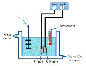
Figure 3. Schematic view of micro-arc oxidation (MAO) process.
