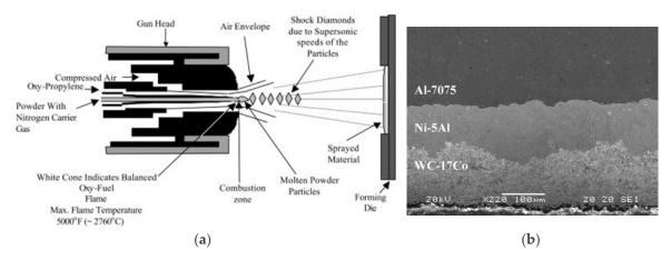
**Figure 9.** (a) Schematic setup of a high-velocity oxy-fuel (HVOF) coating system [89] and (b) cross-section SEM micrograph of HVOF-sprayed multilayer coating on Al7075-T7351 plates [87].
