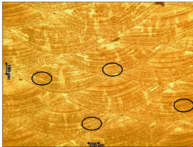
Figure 8. Multilayered build #7 (low P_f:T_s ), considerable re-melting which leads to microsegregation (black circles), and larger grains, Vickers: 213 \pm 14 .
