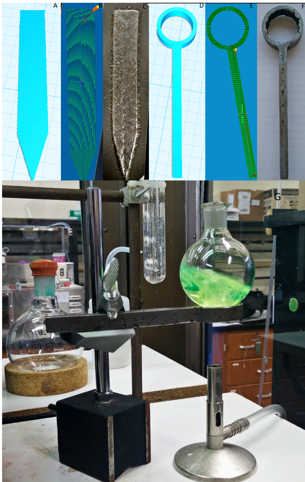
Figure 3. (A) 3-D model; (B) toolpath; (C) metal 3-D printed part on substrate; (D) 3-D model; (E) toolpath; (F) metal 3-D printed part; and (G) ring support used in a chemistry laboratory.
