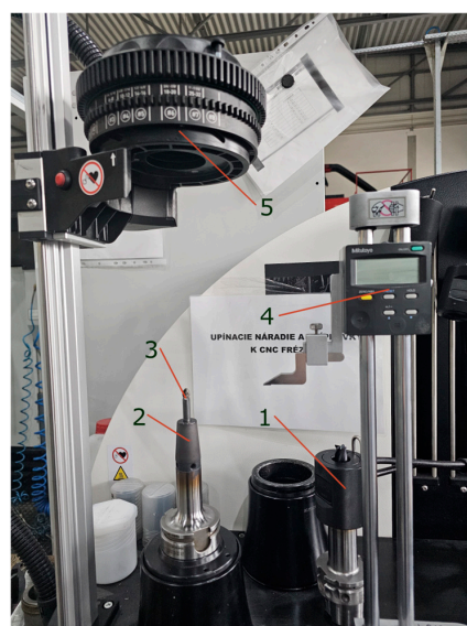
Figure 4. Cutting tool clamping station: 1—cooling element, 2—cutting tool holder, 3—cutting tool, 4—adjustable height meter, and 5—heating element.
