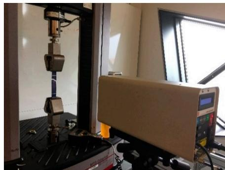
**Figure 9.** Tensile testing of the printed specimen.
