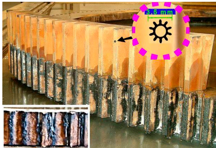
Figure 8. Two AWJ-cut gears with vastly different size and thickness.
