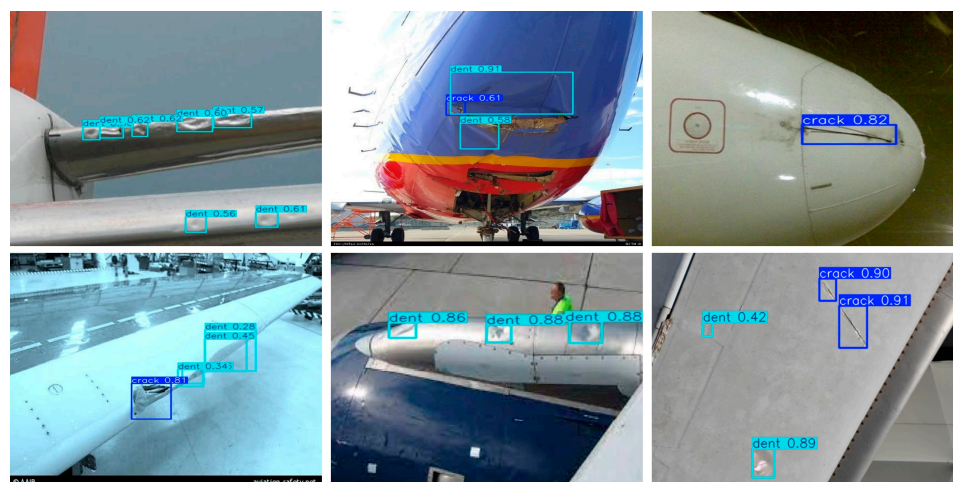
Figure 12. Example of defect detection results.
