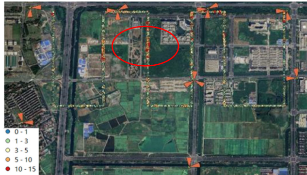
Figure 16. Multi-BS sensing test results at the altitude of 100 m–positioning accuracy.
