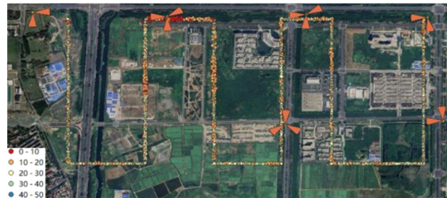
Figure 17. Multi-BS sensing test results at the altitude of 300 m–SNR.
