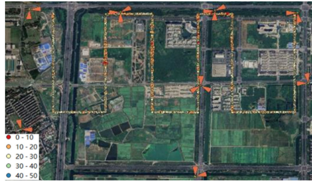
Figure 15. Multi-BS sensing test results at the altitude of 100 m–SNR.
