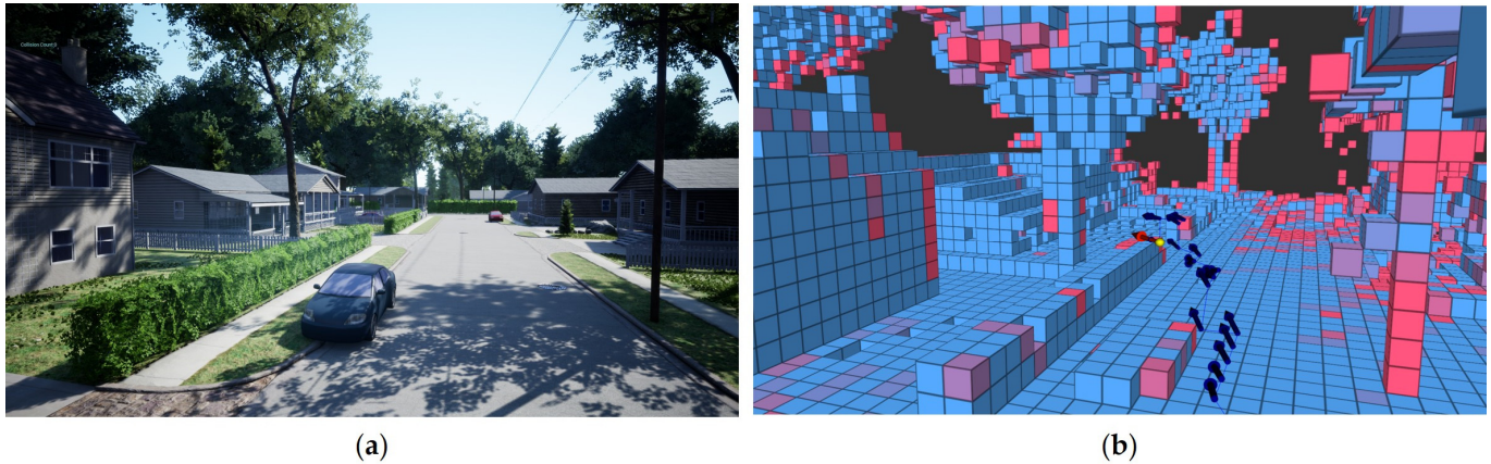
Figure 6. Snapshot of AirSimNH environment mapping result using depth images acquired from AirSim. (a) RGB image; (b) occupancy grid map visualized in rviz. Different color blocks represent known occupied space: blue means higher occupancy certainty; red means lower.
