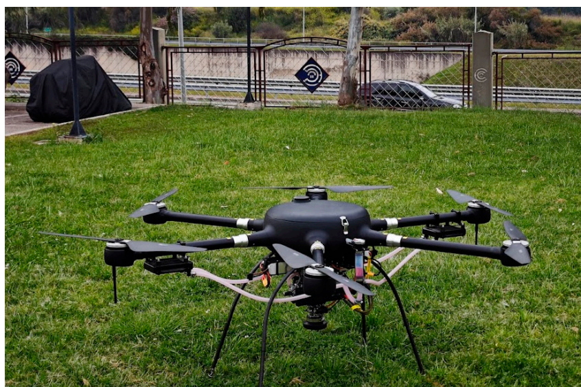
Figure 8. The Hellenic Open University YANGDA YD6-1600L hybrid UAV used for field testing. The platform offers 2–3 h endurance, supports a 3–5 kg payload, and can carry a multigas CO 2 sensor package for gas measurements.
