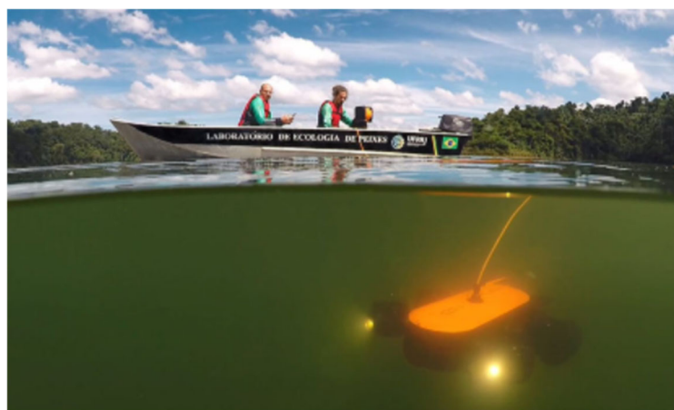
Figure 11. ROV model Genneino T1 used for monitoring fish in reservoirs [116].
