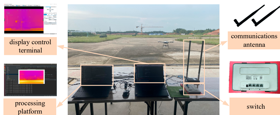
Figure 15. Schematic diagram of data processing platform structure.
