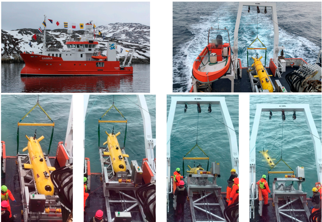
Figure 11. Research vessel R/V Sanna and the LARS system installed on the deck ( top ). The launch and recovery system (LARS) process is depicted showing the procedures involved in deploying and retrieving the vehicle during missions ( bottom ).
