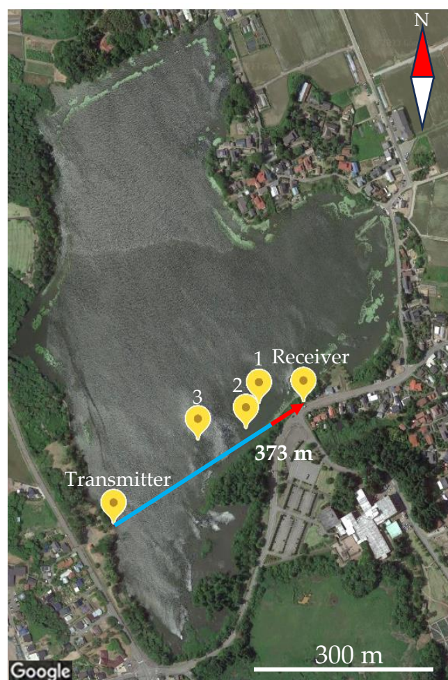
Figure 19. Locations of wireless water quality monitoring system for bypassing relay test (Ogata Pond on 27 September 2022): Transmitter, transmitter drone (landed on the water and was fixed by mooring from shore); 1–3, locations where the relayer drone was placed; Receiver, receiver on a tripod. Red arrow indicates the wireless communication path blocked by shoreline vegetation.
