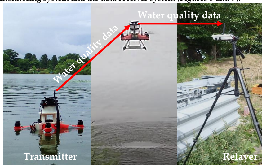
Figure 8. Scheme of the wireless data relay tests. The transmitter drone measured surface water quality data and transmitted the data. The relayer drone relayed the data to a receiver. The receiver received the data.
