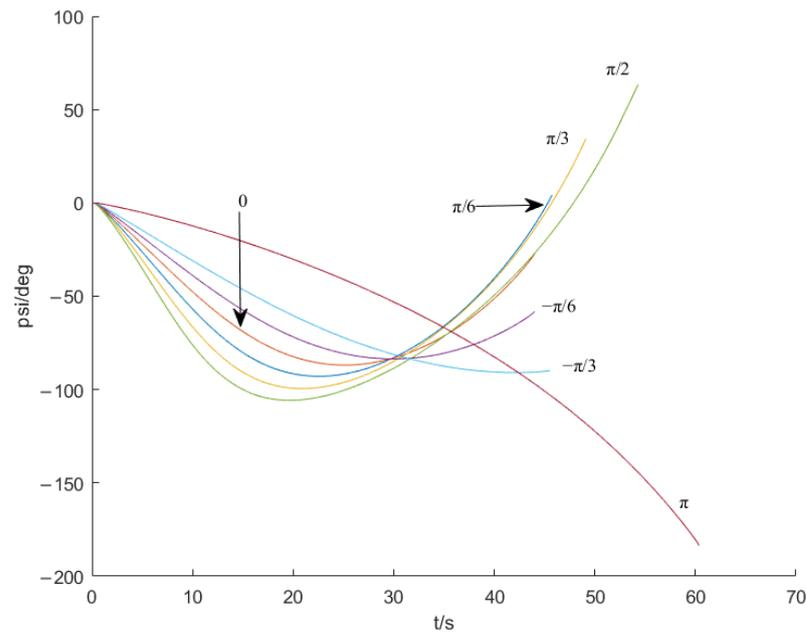
**Figure 8.** The trajectory inclination angle result graph under different angle constraints.
