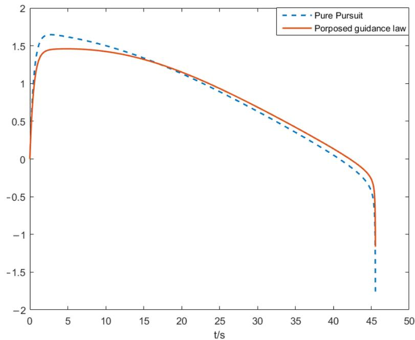
Figure 10. The overload comparison diagram of the two methods.
