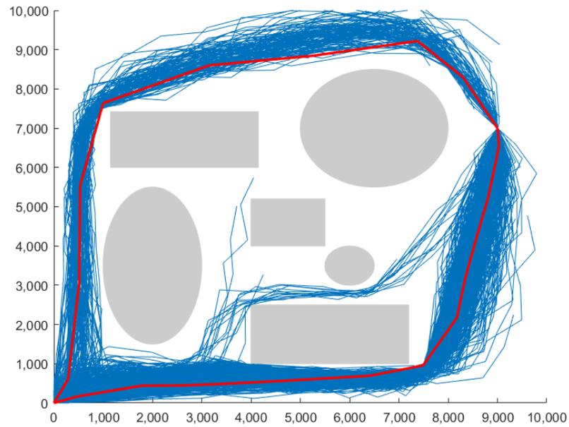
Figure 5. Path planning based on DB-RRT\* algorithm.
