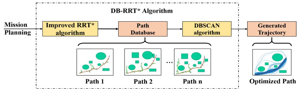
Figure 1. Flow chart of the DB-RRT\* algorithm.
