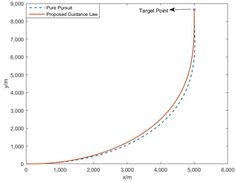
Figure 9. The trajectory comparison diagram of the two methods.
