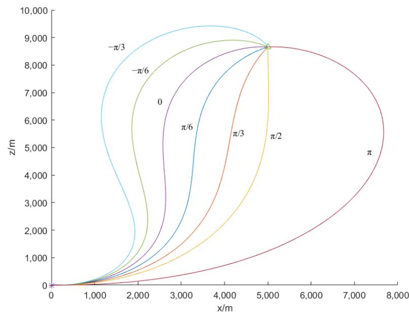
Figure 6. The motion graph in the two-dimensional plane under different angle constraints.
