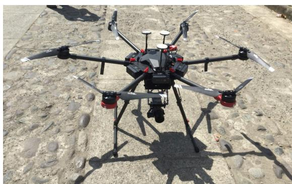
**Figure 2.** Hexacopter UAV model, Matrice 600 DJI (DJI® Austin, TX, USA).
