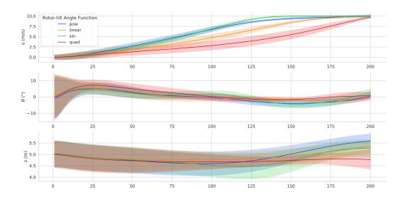
Figure 12. The simulation results of the TRUAV with different rotor tilt angle rates.
