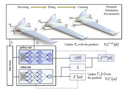
**Figure 3.** Schematic diagram of our process. In the simulation, the agent learns the continuous control of the attitude with the PPO algorithm during the transition process.
