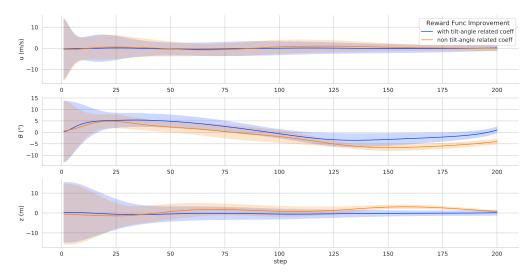
Figure 8. The performance of the UAV while training with/without the tilt-angle-related attitude cost.
