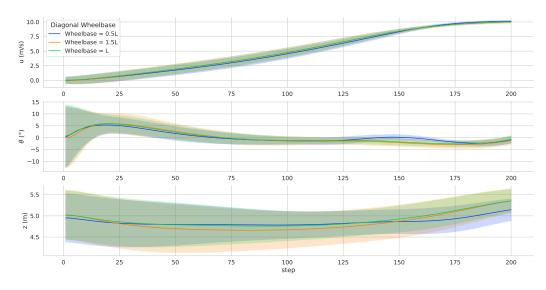
Figure 10. The simulation results of the TRUAV with different diagonal wheelbases.
