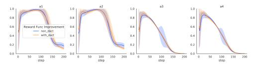
**Figure 7.** The figures are the output of the throttle a = (a1, a2, a3, a4) while training with/without the jitter cost.
