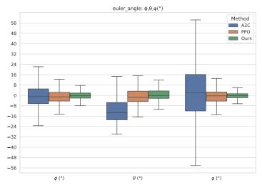
**Figure 13.** The attitude of the TRUAV with different methods at the end of the transition process (200th step). The standard PPO and our proposed method have a better performance at the end of the transition process compared with the standard A2C.
