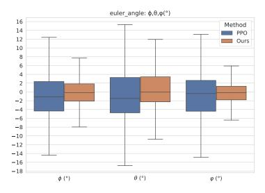
**Figure 15.** The attitude of the TRUAV with different methods at the end of the transition process. Compared with the standard PPO, our proposed method performs better at deviation between attitude angles and desired values.
