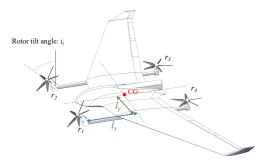
**Figure 2.** The layout of the TRUAV. The front motors  $r_1$  and  $r_2$  can rotate to the horizontal level compared to the fuselage. The rear motors  $r_3$  and  $r_4$  are fixed, and the thrust is vertically upward compared to the fuselage.
