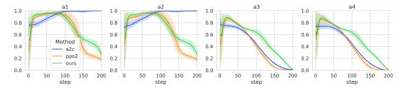
**Figure 14.** The outputs of the controllers with different methods. In terms of energy efficiency, the standard PPO and our proposed method have a better performance at the end of the transition process compared with the A2C. Our proposed algorithm reduces the deviation between attitude angles and desired values at a slightly larger energy cost compared with the standard PPO.
