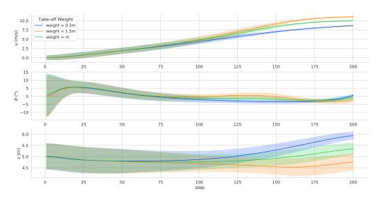
**Figure 9.** The simulation results of the TRUAV with different take-off weights. u(m/s) is the x-axis speed,  $\theta(^{\circ})$  is the pitch angle and z(m) is the altitude of the TRUAV during the transition process.
