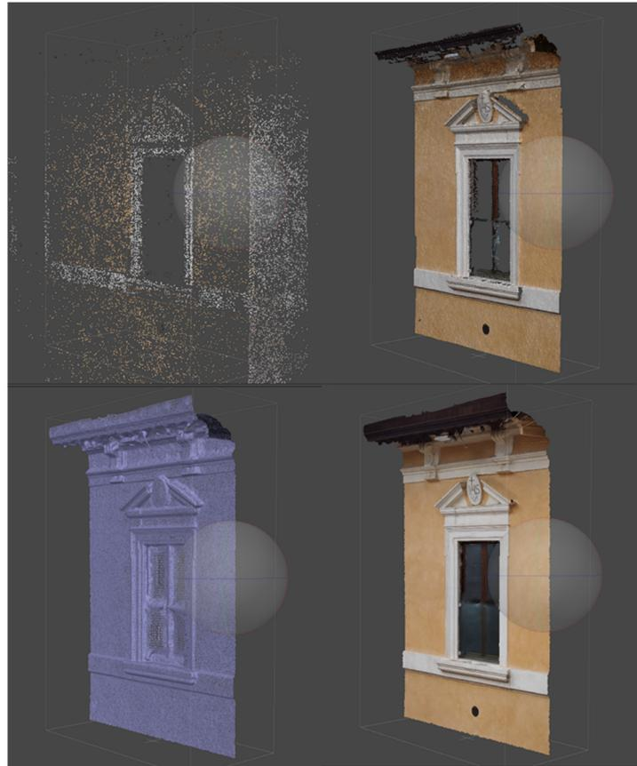
**Figure 2.** Processing of photogrammetric drone survey: sparse cloud, dense cloud, mesh model, textured mesh model.
