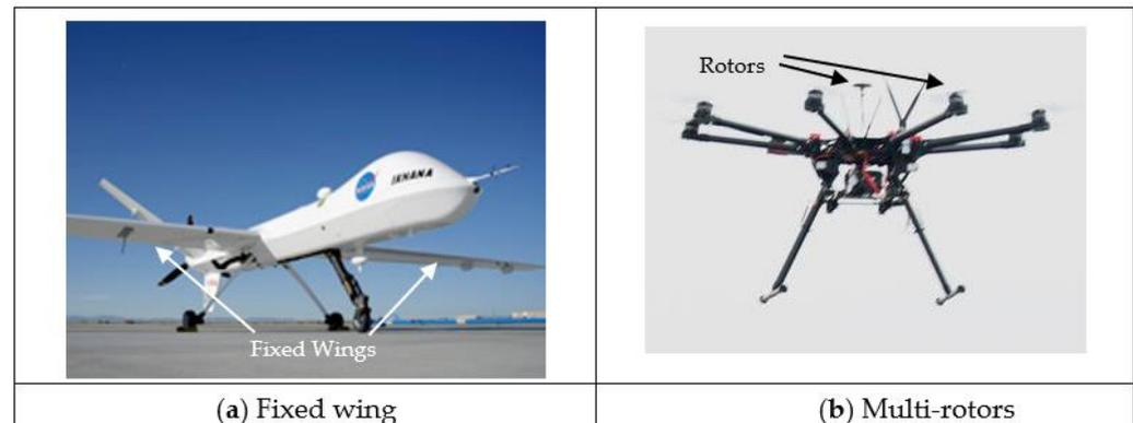
**Figure 2.** Commonly used UAV. (a) Fixed-wing UAV [29] and (b) multi-rotors UAV [30].
