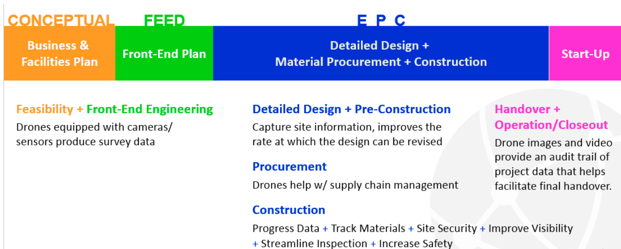
Figure 2. The role of drones throughout a project life cycle.
