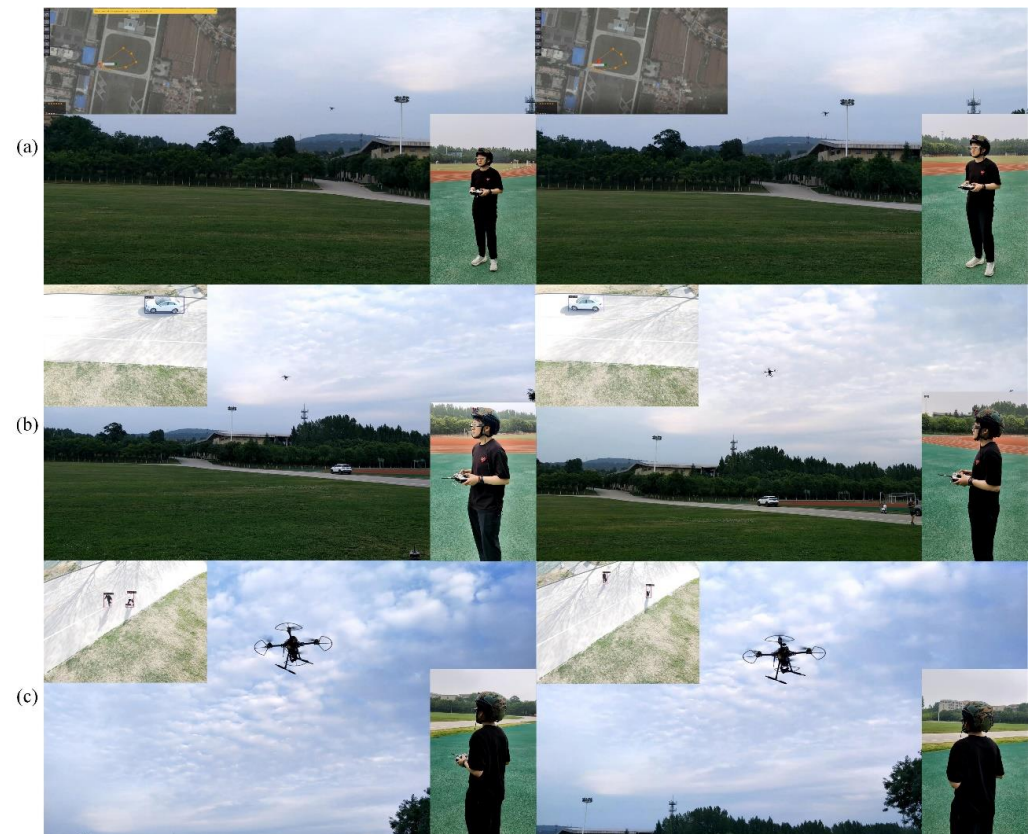
Figure 16. The VisionICE system workflow. (a) UAV takes off and patrols according to the specified route. (b) UAV detects vehicle. (c) UAV detects pedestrians.
