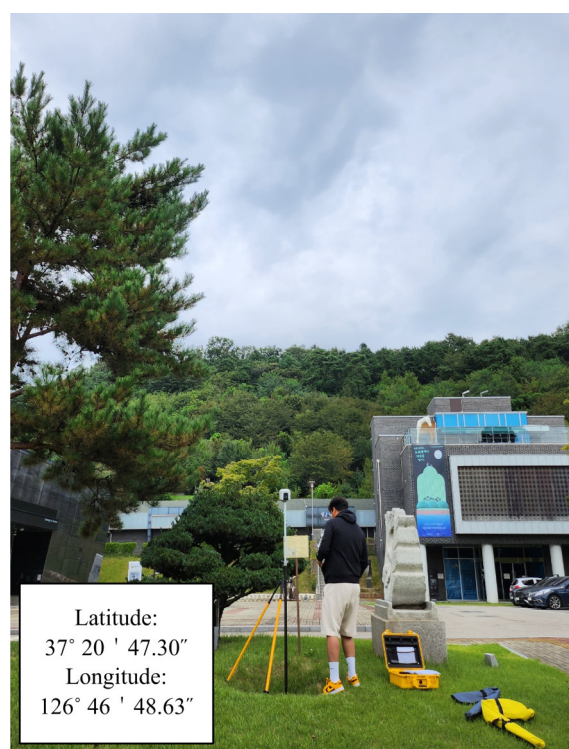
Figure 4. External virtual reference station (VRS)-GNSS survey for site calibration.
