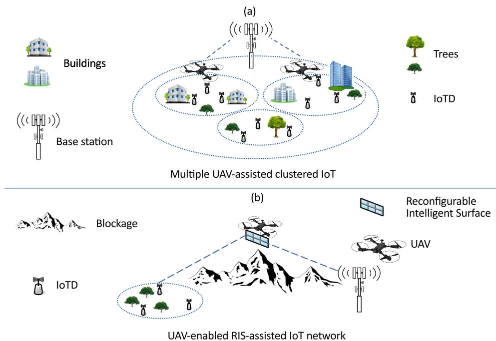
**Figure 13.** Illustrative architecture for multiple-UAV-assisted clustered IoT (a) and UAV-RIS-assisted IoT (b) based on [8,9], respectively.
