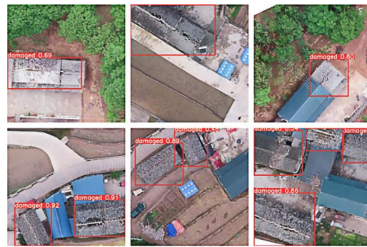
Figure 25. YOLOv5s-ViT-BiFPN algorithm for detecting damaged houses [135].
