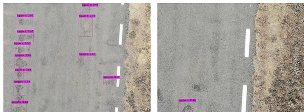
Figure 18. Road damage detection results [77].
