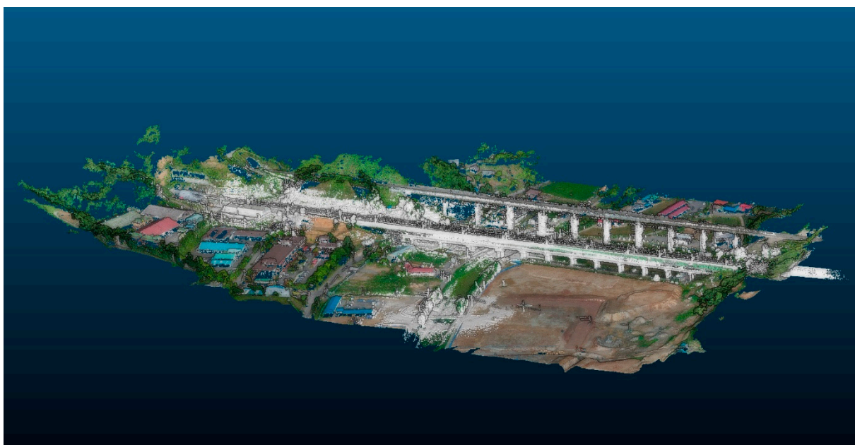
Figure 4. Merging of point cloud data acquired by a UAV and handheld LiDAR sensor.
