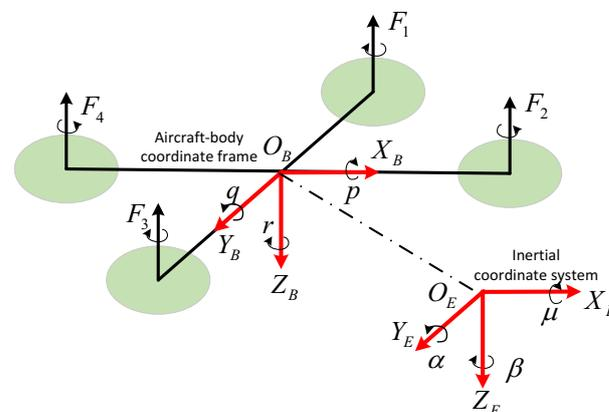
Figure 1. Three-dimensional view of quadrotor attitude definition.
