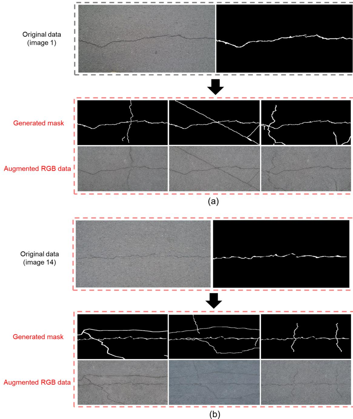
**Figure 6.** Examples of augmented data from specific images in dataset 1: (a) image 1, (b) image 14.
