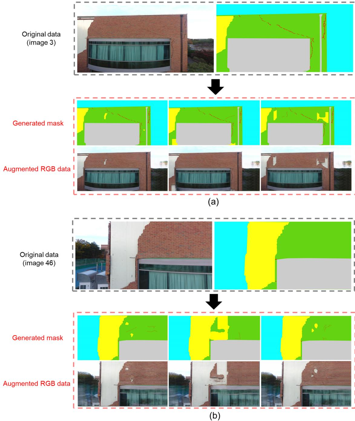
Figure 8. Examples of augmented data from specific images in dataset 2: (a) image 3, (b) image 46.
