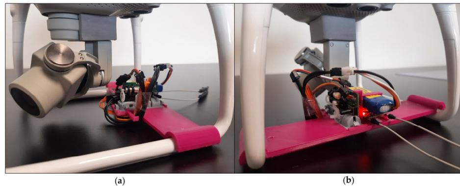
**Figure 1.** Payload system attached to a DJI<sup>®</sup> Phantom 4 RTK. View from left (a) and view from behind (b).
