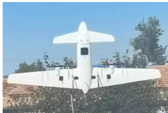
Figure 2. The tail-seat vertical takeoff and landing fixed-wing UAV platform used in this study.
