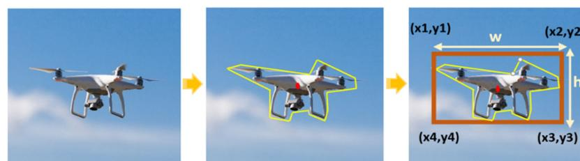
**Figure 6.** The conversion of the polygon to the best-fitted rectangle.
