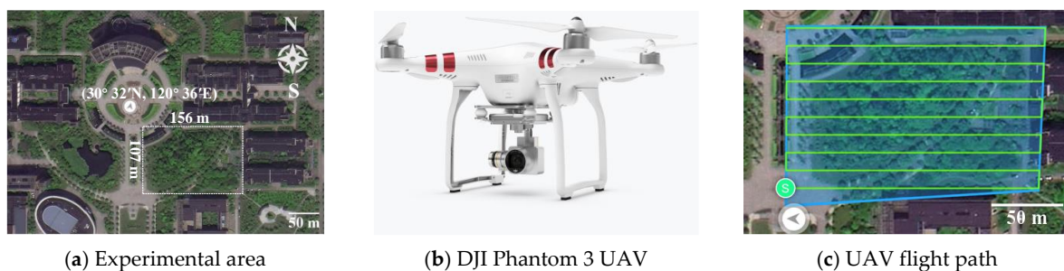
Figure 2. The experimental area and mission design. (a) The rectangular area marked by white lines represents the experimental area. (b) The DJI quad-rotor aerial photography UAV that was used in the experiment. (c) The flight path design of the UAV.
